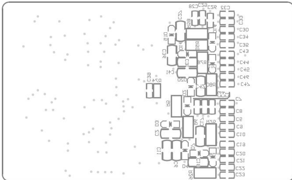
Bottom Layout of BMS board 2
