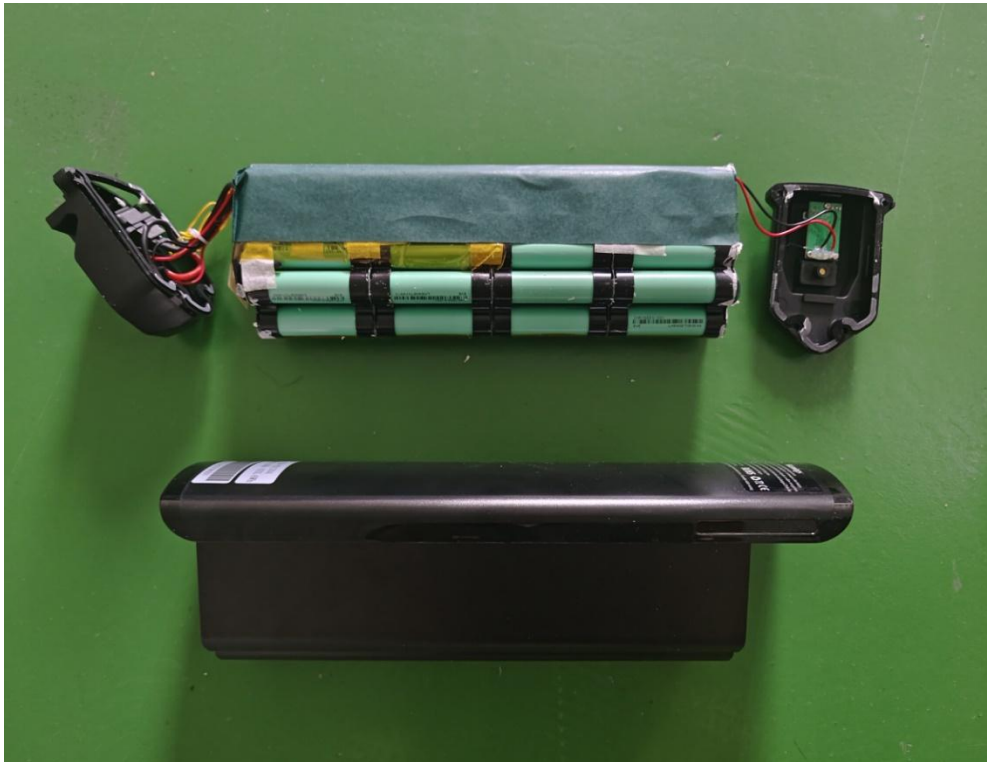
Internal view 1 of battery pack
