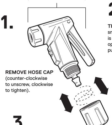
THREAD HOSE THROUGH CAP smaller diameter cap opening
