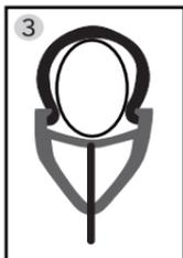
Starting at the valve stem, push second bead onto rim.
