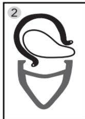
Place partially inflated tube inside tire casing and straightened valve stem.
