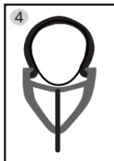
Inflate tire to recommended pressure and test beads for integrity.
