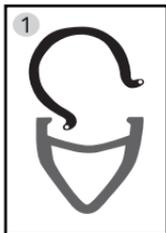
Insert one side or bead of tire into rim.
